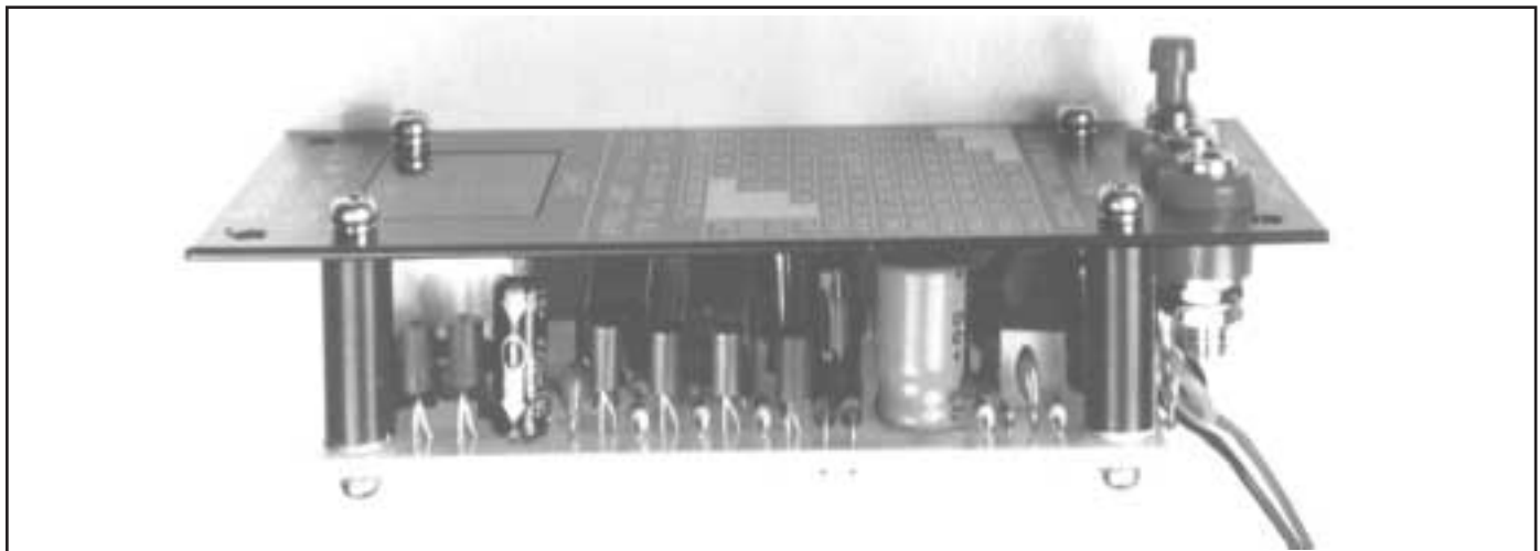
The display window (perspex) is inserted into the panel cut-out from inside the flush with the front panel.
